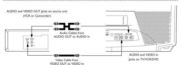
Make the connections shown above. Use audio and video cables (not supplied). Connect the source unit (VCR or Camcorder) to a power source after connections are made.
